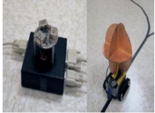
Figure 5: Left: A Doppler radar for tracking moving targets. Right: Target to be tracked.
