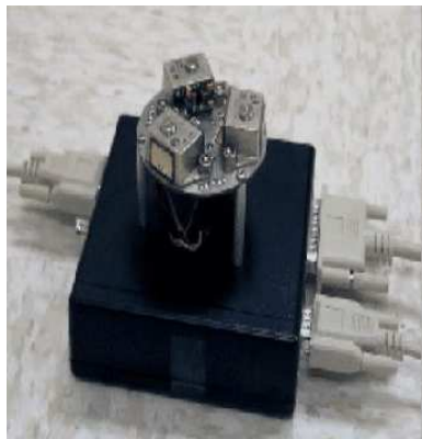
Figure 2.1: A hardware sensor (left) and schematic of nine sensors in a grid layout (right).
