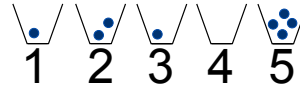
Fig. 6. For a five agent graph and a L = 2 algorithm, up to two of the five bins could receive a ball in each round. A configuration (such as the one shown above) would indicate that agent A_i takes value \lambda_j where there are j balls in the i -th bin. The configuration shown above is reachable by a L = 2 algorithm in 4 rounds, but not in 3 rounds – bin 5 contains 4 balls.
