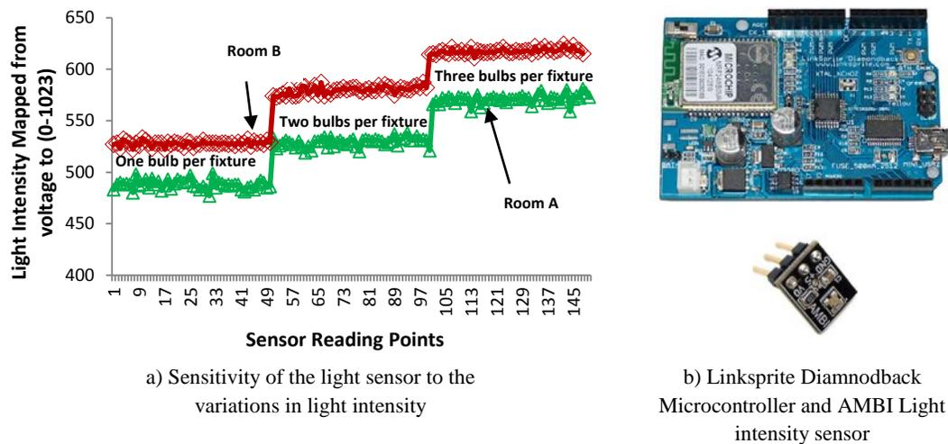
Figure.1 Light intensity sensor components
