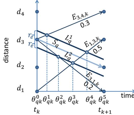
Figure 4.4: An example to show how a target moving from  $d_3$  to  $d_2$  during  $[t_k, t_{k+1}]$  is protected. In a sub-interval  $[\theta_{qk}^r, \theta_{qk}^{r+1}]$ , a patroller either always protects the target or never protects the target. Equivalently, the target is either always within the protective circle of a patroller or always outside the circle.
