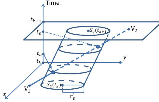
Figure 4.10: An illustration of the calculation of intersection points in the two-dimensional setting. The  $x$  and  $y$  axes indicates the position in 2-D and the  $z$  axis is the time. To simplify the illustration,  $z$  starts from time  $t_k$ . In this example, there are two intersection points occurring at time points  $t_a$  and  $t_b$ .
