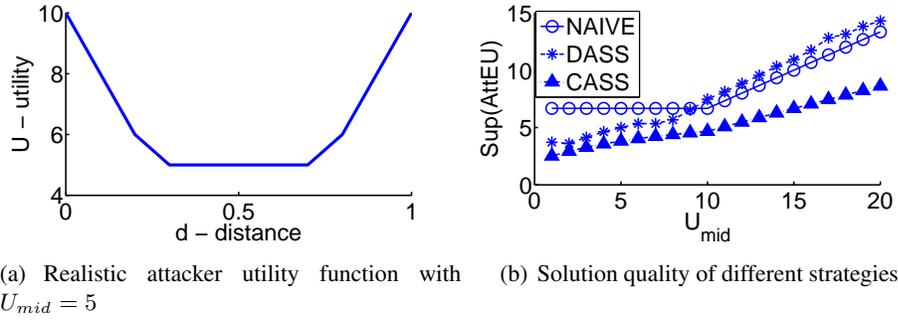
Figure 4.13: Performance under different realistic utility function settings. The utility function is U-shape or inverse U-shape. The utility around distance 0.5 is denoted as  $U_{mid}$ . We compare the defender strategy given by DASS and CASS with the baseline when  $U_{mid}$  is changing from 1 to 20.
