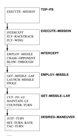
**Figure 10:** LL's problem space hierarchy. Boxes indicate problem spaces, with names in bold to their right. Names within boxes indicate operators available within problem spaces. Italicized names indicate currently selected operators.
