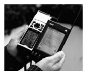
Figure 2: PDA (Palm VII) with GPS device
