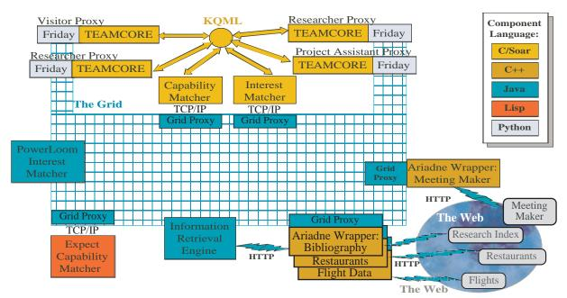
Figure 2: Electric Elves System Architecture
