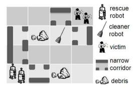
Figure 1: A  $4 \times 4$  Rescue Domain where two rescue robots plan to reach two victims (1089 joint states).
