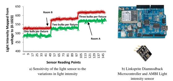
Figure.1 Light intensity sensor components
